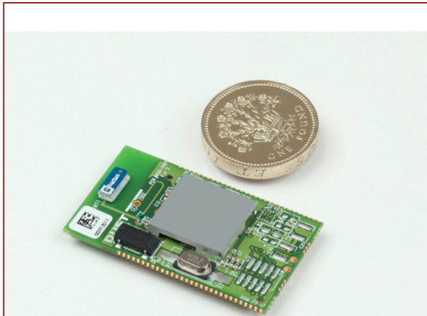
Figure 4: Small TSCH-based wireless nodes, such as the LTP5901-IPM from Linear Technology, deliver 5-10 years of battery life with data reliability > 99.999%
