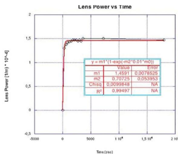
Figure 4: Lens power (YAG)
