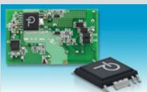
Inside the new device, highly accurate secondary-side direct voltage and current measurements are communicated across the safety isolation barrier using high-speed digital FluxLink technology. This proprietary new feedback technique permits precise control without the need for a bulky optocoupler, while avoiding the performance compromises inherent in primary-side regulation (PSR), such as limited accuracy and efficiency and poor transient response versus no-load consumption.
