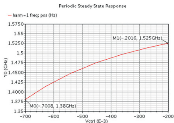
Figure 8: The output frequency versus the control voltage of the QVCO
