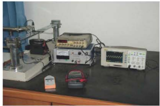
Figure 6: Piezoelectric generator test setup
