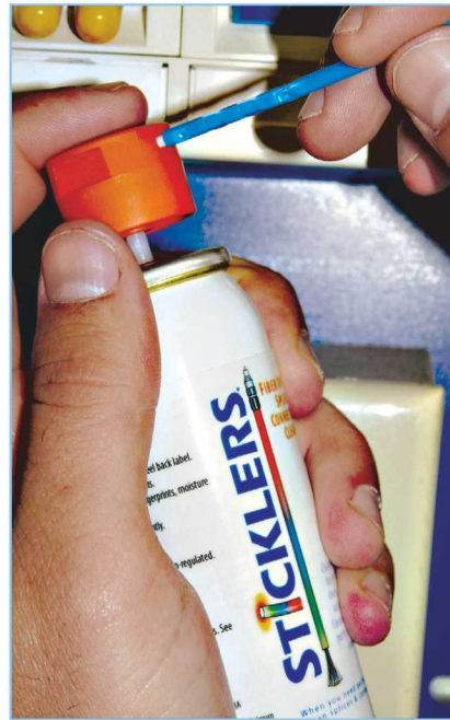
Figure 6: The “wet-dry” cleaning technique is important for cleaning ports, as well as cleaning exposed end-faces. First, a technician dampens a cleaning swab with a nonflammable, fast-drying cleaning fluid. Then he inserts the cleaning tool into the port to ensure no residues remain on the end-face
