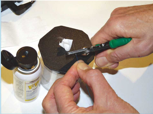
Figure 4: It is absolutely essential the bare fibre be perfectly clean before inserting into a ferrule during connectorisation. Here the operator is preparing to clean with high-quality lint-free wipe that does not contain any glues or cellulose. The cleaning fluid evaporates quickly and the canister cannot be refilled, which ensures the cleaning fluid will remain pure and uncontaminated
