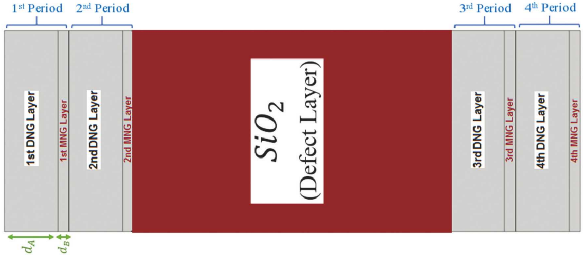
Figure 5: The new compound metamaterial (DNG-MNG-SiO 2 )
