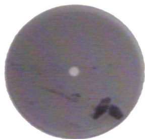
Figure 1: A close-up of a clean end-face, to illustrate the objective of what has to be cleaned
