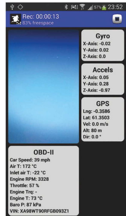
Figure 6: TrackSpy data and video view (the video image is obscured)
