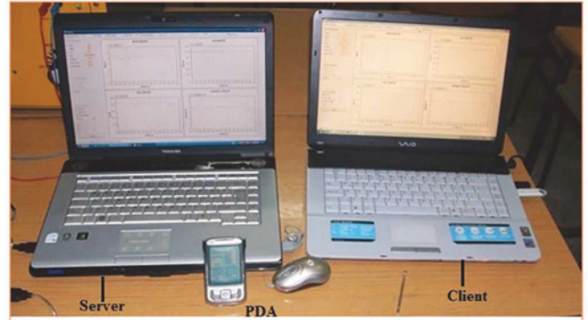
Figure 6: Server and client laptops, and client mobile phone used in the setup
