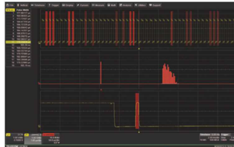
Image 3 - WaveScan allows searching analog, digital or parallel bus signal in a single acquisition using more than 20 different criteria.
