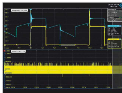
Figure 7: Measurement of the drain-source voltage of a DC/DC converter without high-definition mode. The large noise component in the signal makes reliable results impossible
