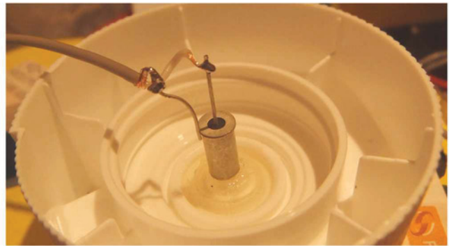
Figure 3: Wiring the screened cable to the tilt switch
