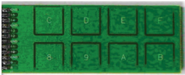
Figure 4: mTouch evaluation kit – 8 pads board
