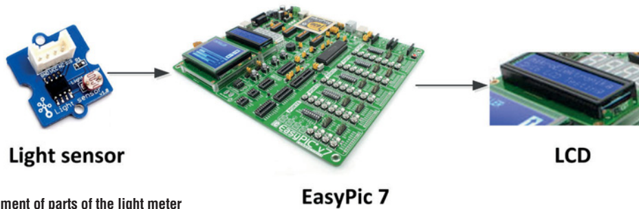
Figure 3: Arrangement of parts of the light meter
