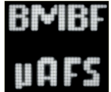
Figure 4: The \mu AFS demonstrator shows 1024 pixels controlled individually with this LED chip
