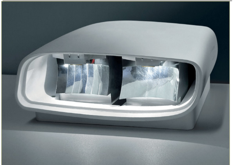
Figure 3: Prototype design of a combined low-beam/high-beam headlamp based on one high-luminance LED each and reflectors measuring just 30mm x 50mm
