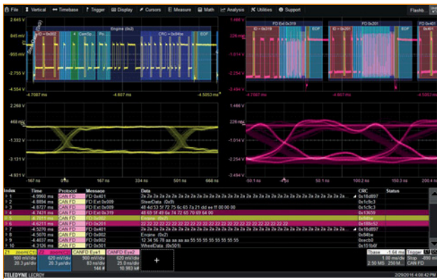
Figure 2: HDO9000 combines Serial Bus Trigger, Decode, Measure/Graph, and as industry first also the Eye Diagrams for the most advanced serial data analysis
