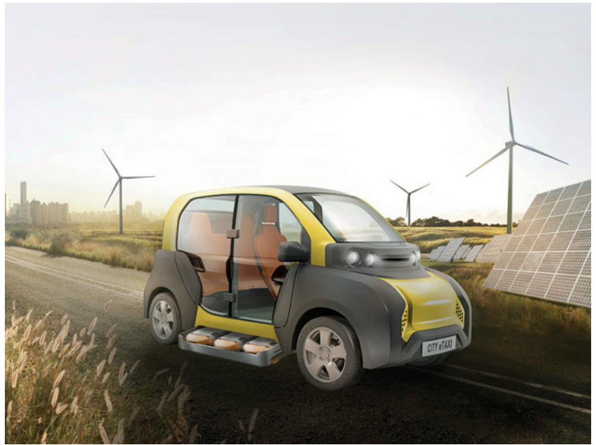
Future electric cars won't need to wait to charge at stations thanks to a set of easily replaceable battery modules, located on the side of the car
