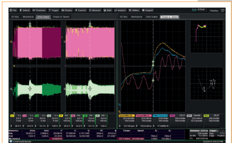
Image 2: This two second capture shows the drive output waveforms on the left and the Torque, Speed and Mechanical Power Waveform per-cycle values over time are shown to the right
