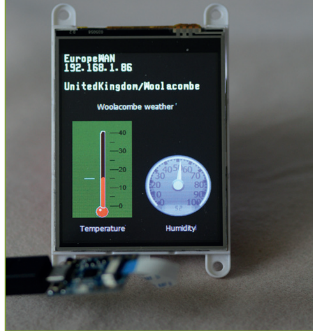
Figure 6: gen4 Internet of Displays module showing the Weather Underground weather observations
