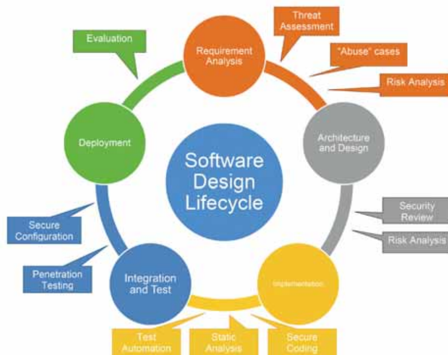
Figure 1: Security processes superimposed over the software development lifecycle
