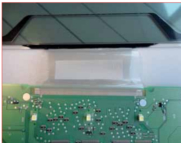
Figure 4: Heat-seal bonding in a display FPC-PCB
