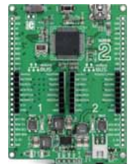
Figure 6: The Clicker 2 for PIC18FJ board
