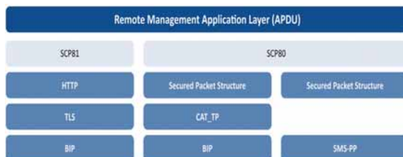
Figure 7: Remote APDUs using secure channel protocols
