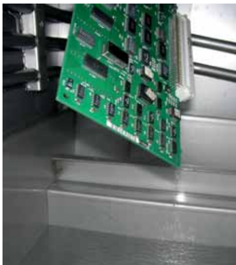
Solvent run-off from PCB undergoing vapour degassing
