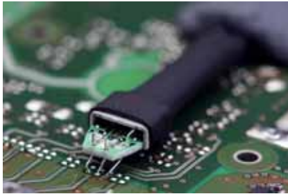
Figure 6: Using the R&S RT-ZMA10 solder-in tip module to contact a high-speed interface
