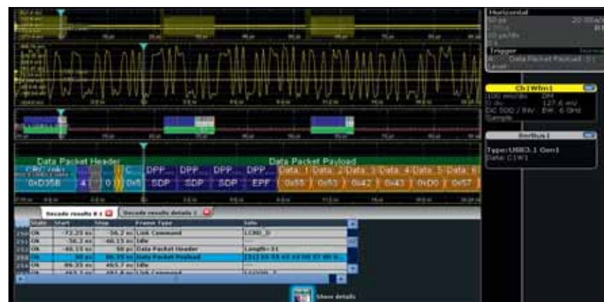
Figure 9: Configuring the trigger type to be a data packet header in line with USB 3.1 Gen 1
