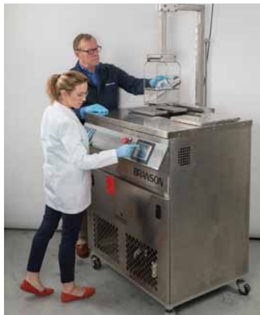
Loading parts into a vapour degreaser
