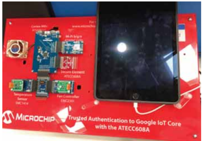
Figure 3: The Google IoT core demo of the ATECC608 secure element
