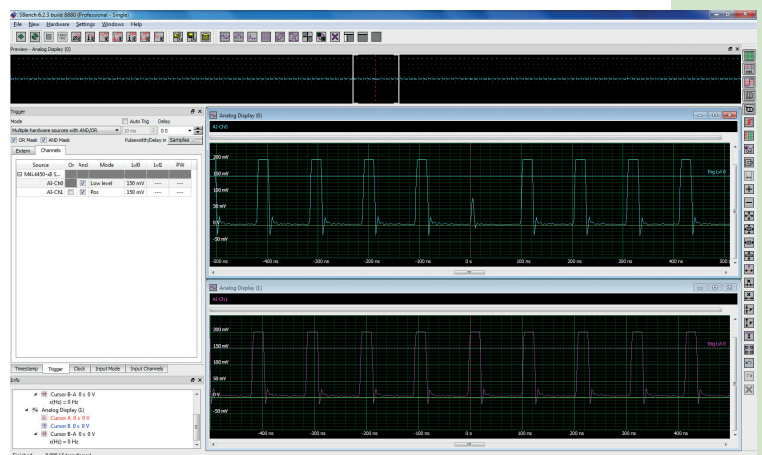
Figure 5: Another example of using the AND trigger function with an inverted logic element (low-level mode on CH0), which triggers when a missing pulse occurs in CH0 compared with the pulse train on CH1
