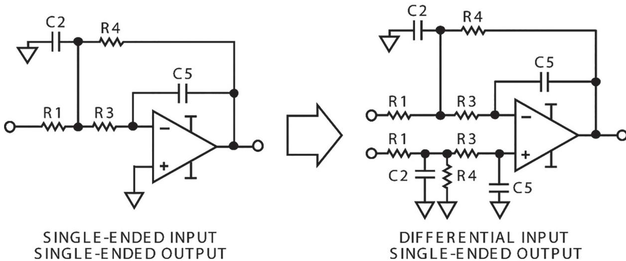
Figure 5: Second-order multiple feedback (mfb) filter
