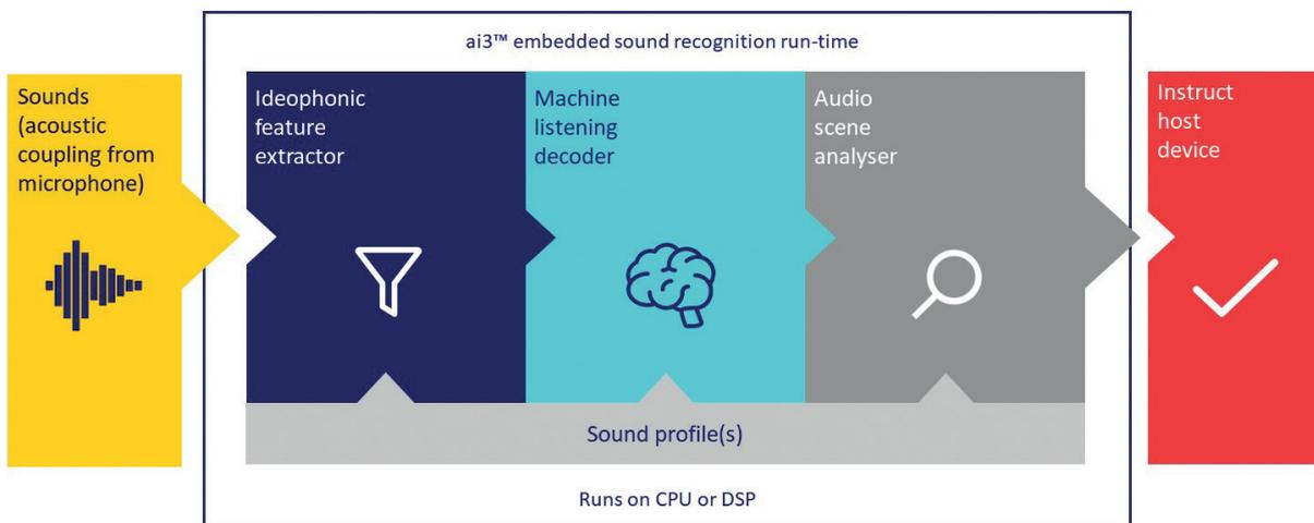
Figure 1: Block diagram of the ai3 sound recognition engine
