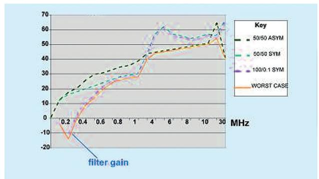
Figure 3: Deriving a reliable filter attenuation curve from manufacturer's data
