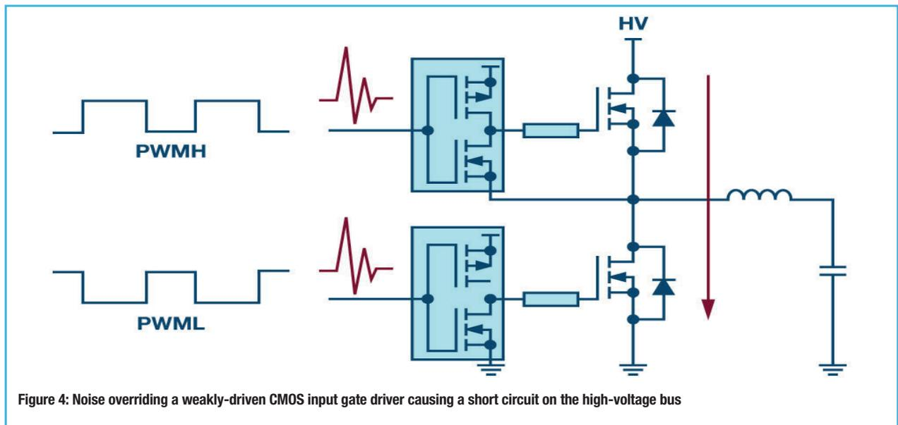
Figure 4: Noise overriding a weakly-driven CMOS input gate driver causing a short circuit on the high-voltage bus
