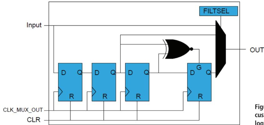
Figure 1: Filter of a custom configurable logic (CCL)
