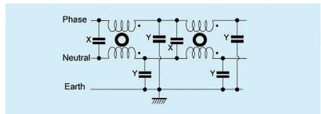
Figure 2: A typical two-stage mains filter
