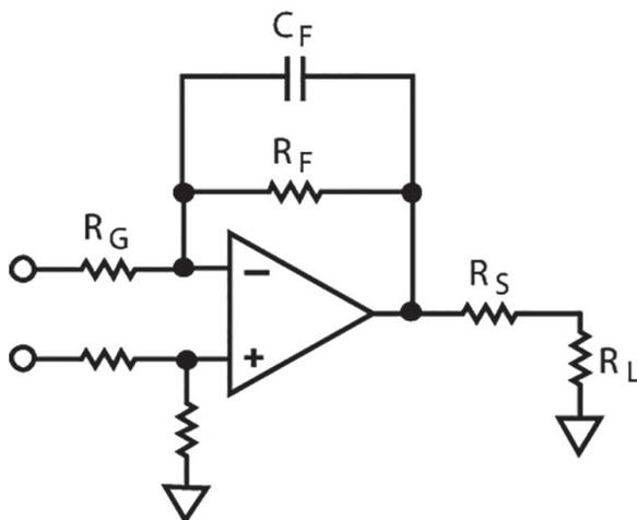
Figure 4: Differential single-ended circuit
