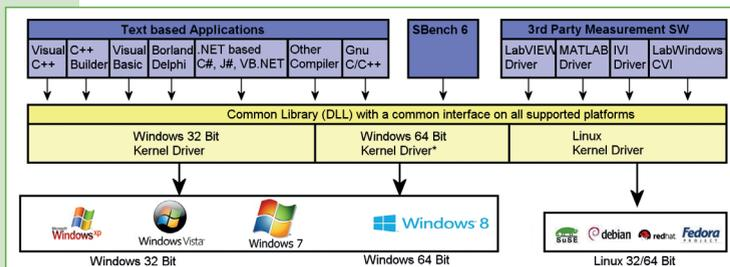
**Figure 1: The digitiser device driver supports commonly-used operating systems while providing a common interface for universally-used programming languages and third-party analysis and control software**
