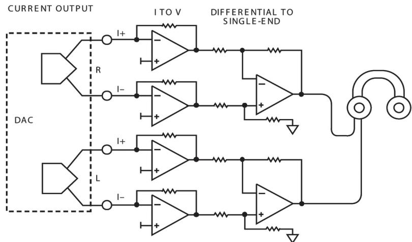
Figure 2: Current output configuration
