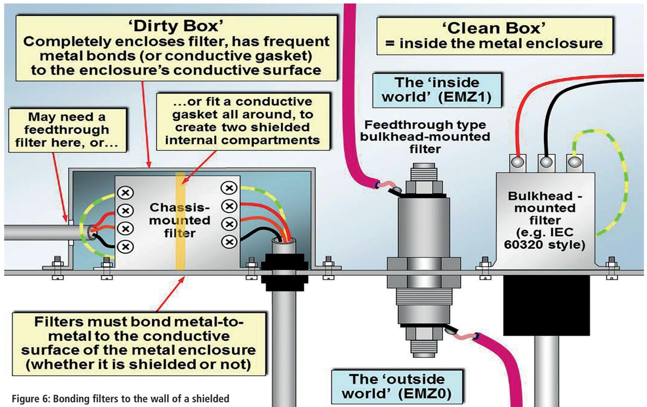
Figure 6: Bonding filters to the wall of a shielded enclosure
