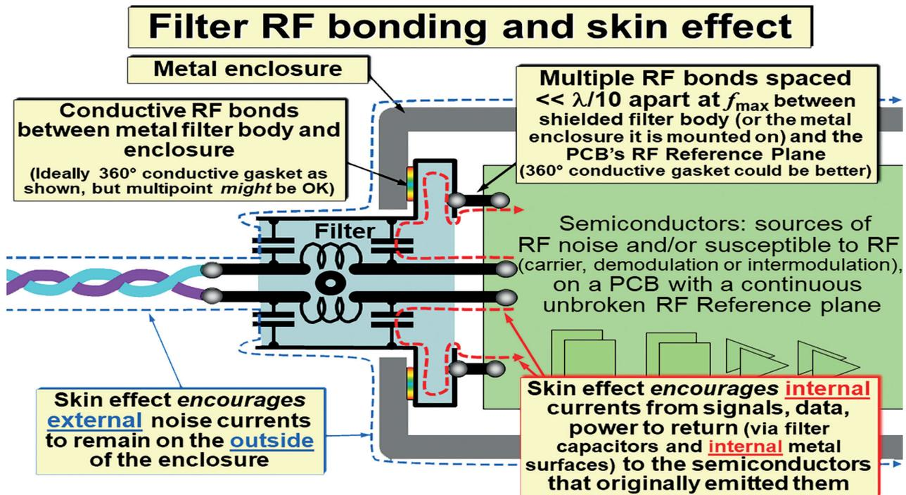
Figure 5: Keeping internal currents inside and external ones outside
