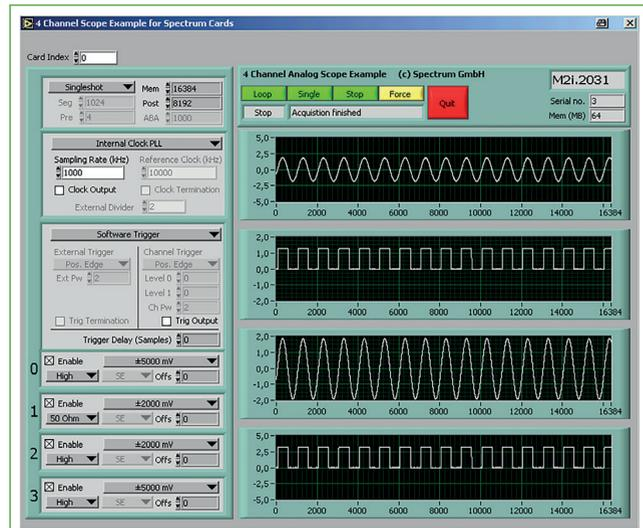
Figure 3: The virtual front panel of a LabVIEW example using the digitiser's analogue acquisition channels as a four-channel oscilloscope
