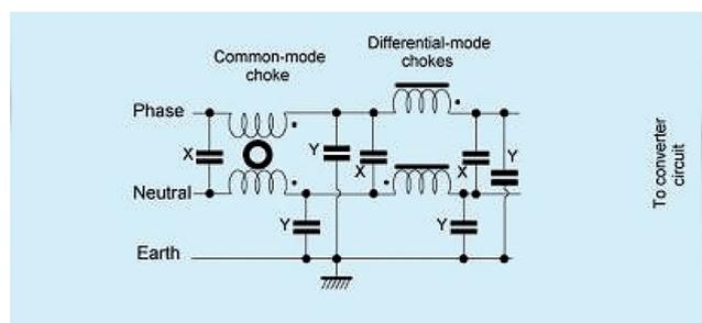
Figure 4: Example of mains filter for a switching power converter
