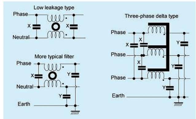
Figure 1: Some typical single-stage mains filters
