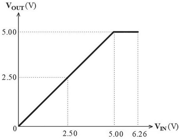
Figure 3: V<sub>OUT</sub> vs V<sub>IN</sub> for the 0-5V analogue input module 1 of Figure 1
