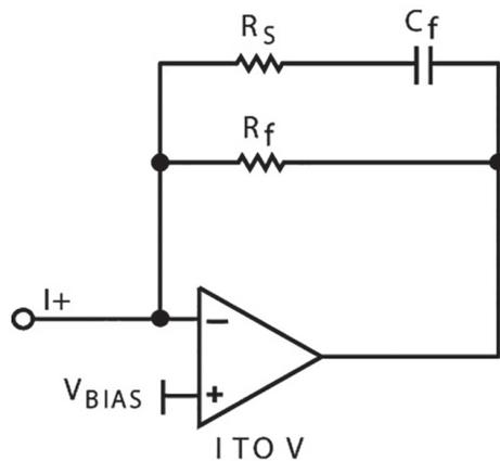
Figure 3: I-to-V stage
