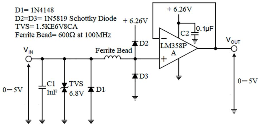
Figure 1: Schematic 0-5V analogue input module 1 to be used with an ADC input of a 5V microcontroller
