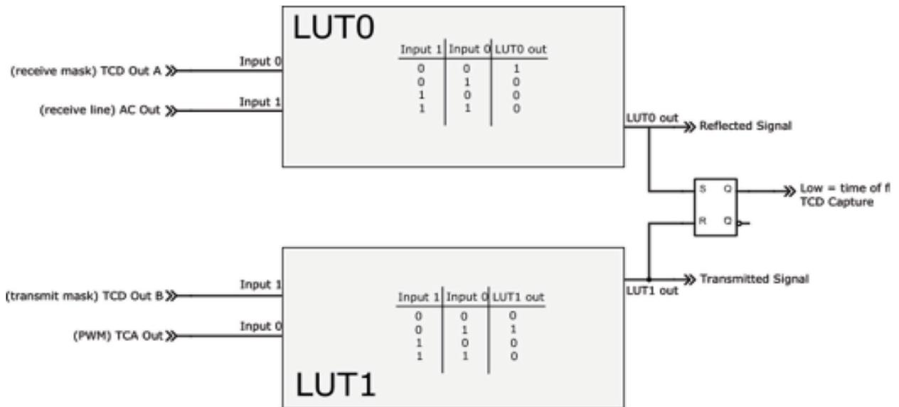
Figure 6: Measuring an ultrasonic signal’s time-of-flight
