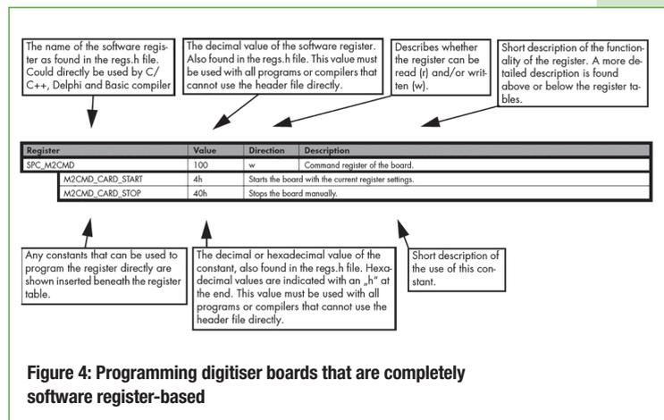
Figure 4: Programming digitiser boards that are completely software register-based
