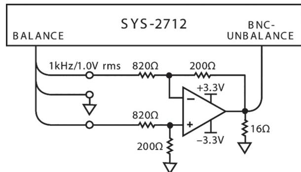
Figure 6: THD + N test with 16 $\Omega$  load
