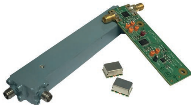
Figure 3: A connectorised directional coupler, surface-mount directional coupler and ADL5920 integrated IC with directional bridge and dual rms detectors
